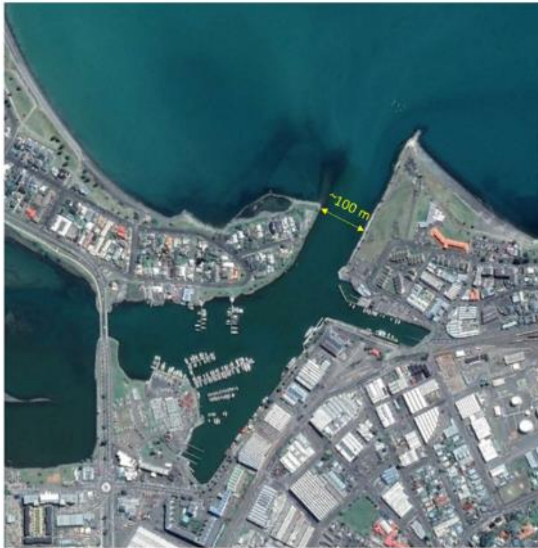
Figure 14: Approximate location and length of storm surge barrier (Beya and Asmat, 2020).
