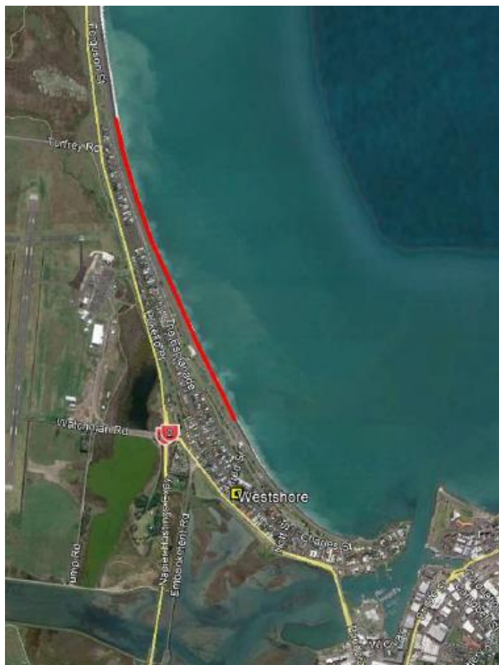
Figure 7: Approximate areas of the Westshore priority unit where an extension to the existing gravel barriers is required (Beya and Asmat, 2019).
