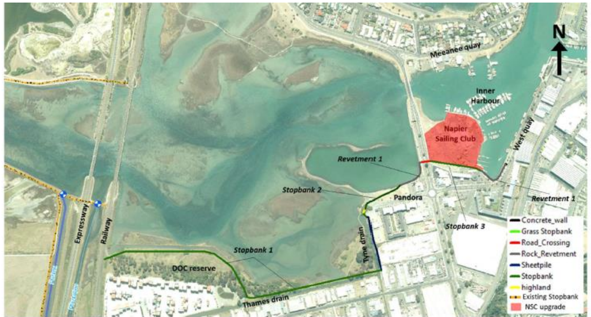
Figure 10: Layout design for the proposed flood defences in the Pandora Priority Unit (Beya and Asmat, 2020).
