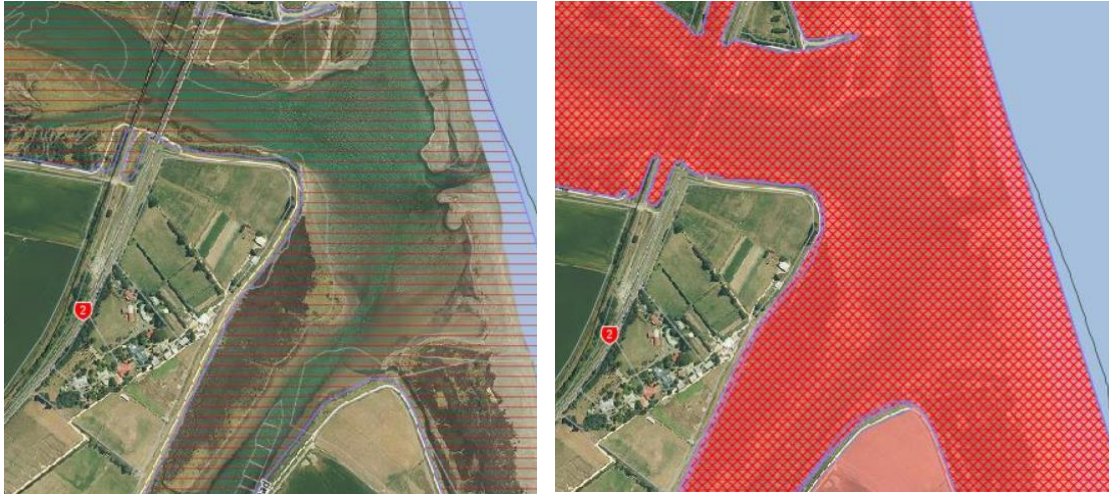
Figure 8 Comparison of sea-borne flooding in a 1:100 AEP event – “Present” with 2120 scenario (right) suggests that Hohepa site continues to remain protected by the stop-bank system from coastal inundation
