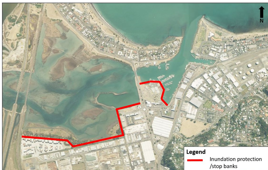
Indicative inundation protection locations at Pandora.
